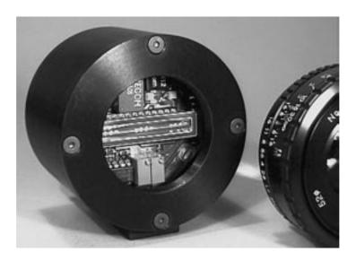
The cameras are housed in a round case (Ø70 x 53 mm, wheight 310g - without case 50g) with M42-mount for the connection of standard lenses.
