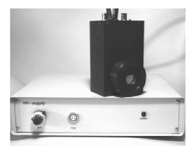
Intensifiers with double or single MCP's (MCP: microchannel plate) are available: They are delivered from different manufacturers (DEP or Proxitronic) with 18 or 25 mm screen diameter.
